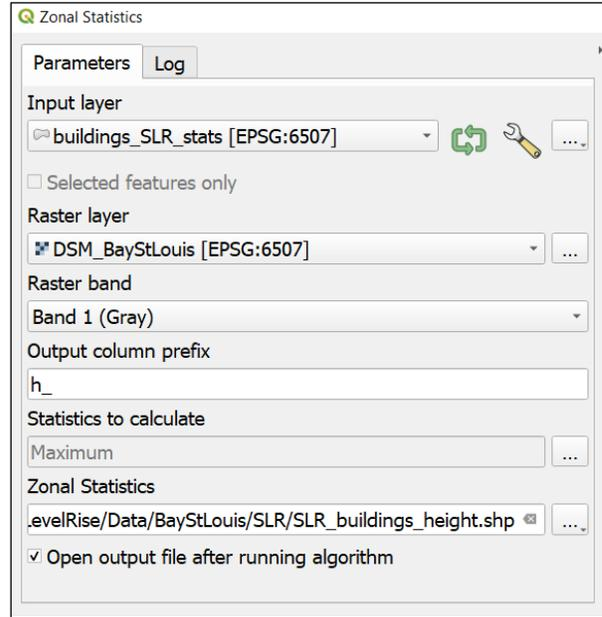
Fig. 2. Running zonal statistics on DSM allows us to assign roof elevation to building layers.
