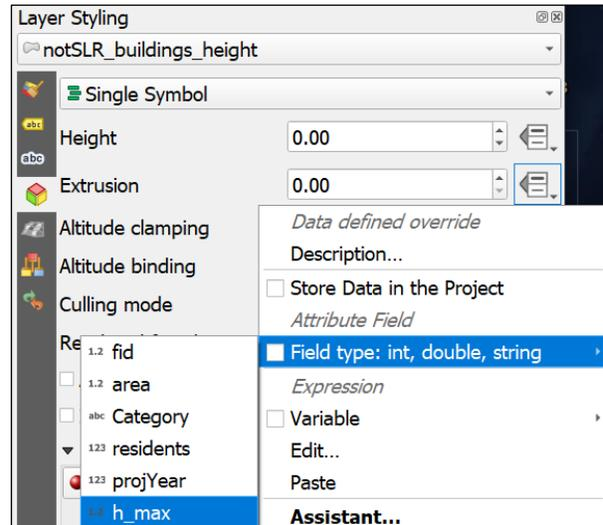
Fig. 5. 3D extrusion setting allows the vertical shift of the features in the 3D map view.
