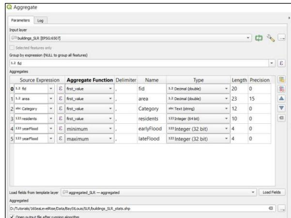
Fig. 3. Aggregating allows to grab multiple features into one geometry, following a group by expression.
