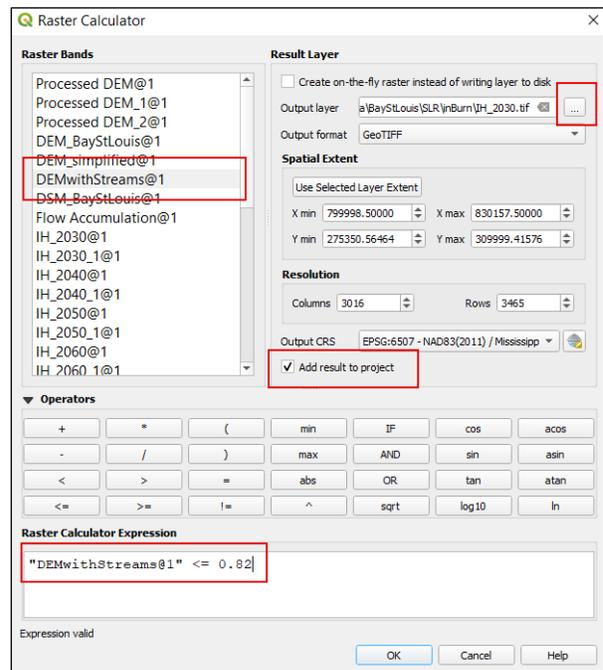
**Fig. 1.** Raster calculator setting for the 2030 SLR projection.
