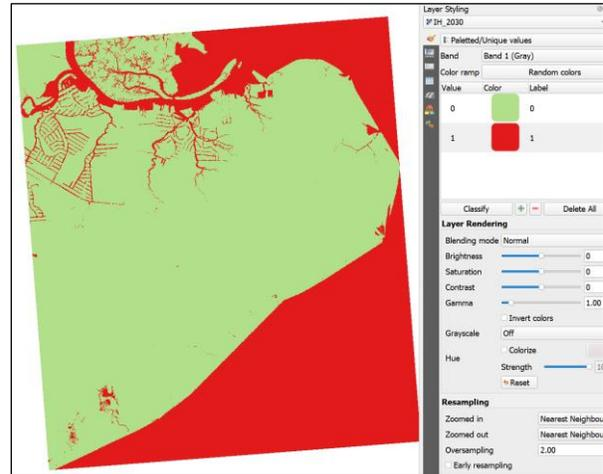
Fig. 2. The output raster is true-false classified, where flooded cells are marked with the value of 1.
