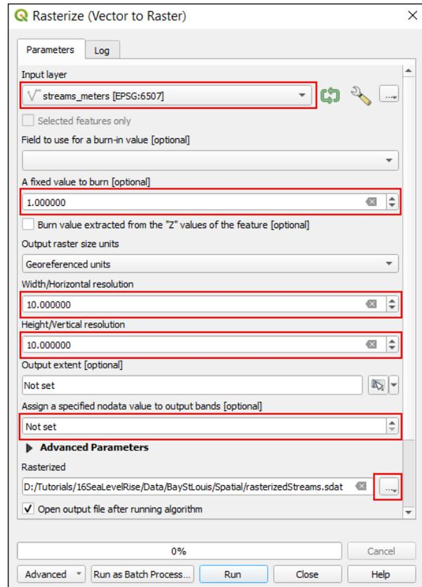
Fig. 2. Rasterize tool allows to change vector data to raster.
