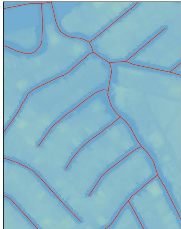
Fig. 5. Vector streams (in red) and the stream network burned in DEM.
