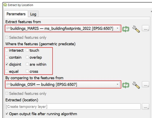
Fig. 3. Using spatial predicates allows to quickly organize data between two layers based on their spatial relation.
