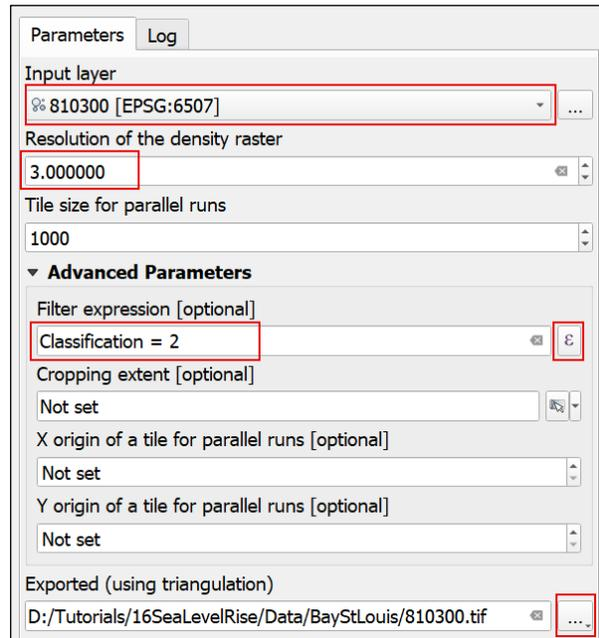
Fig. 6. Settings used in QGIS to compute DEM with empty cells filled.
