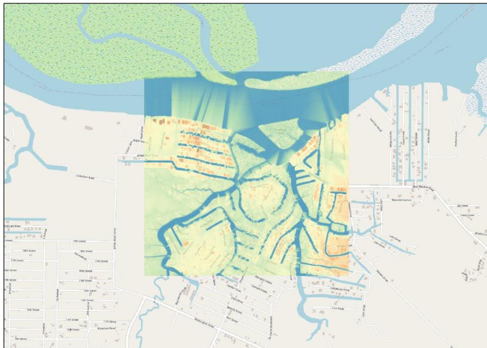
**Fig. 5.** Using OpenStreetMap as a background layers helps verifying if the resulting DEM is correctly positioned.
