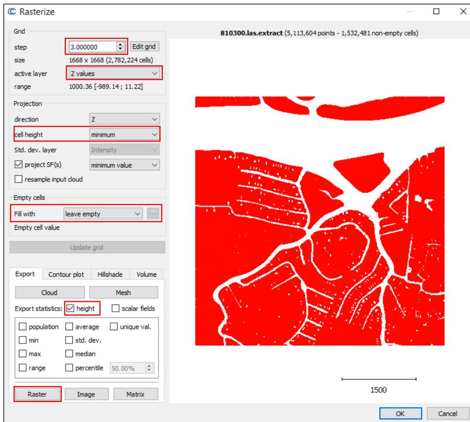
Fig. 4. Rasterization settings allow for different ways to create raster and handle missing data.
