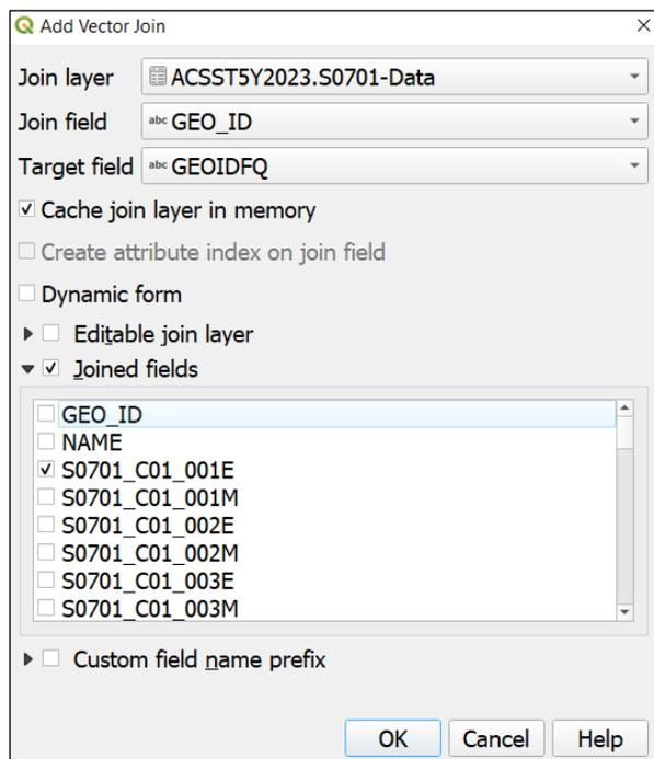
Fig. 4. Join settings in QGIS allows to define table columns to be joined as attributes to the spatial layer.
