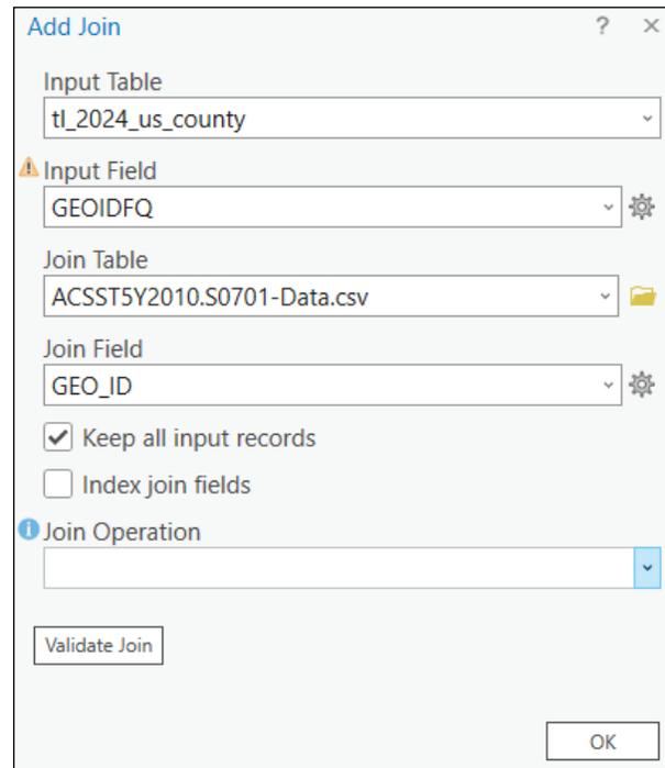
Fig. 3. ArcGIS Pro settings in batch process allow to choose the parameter that will change in each batch.
